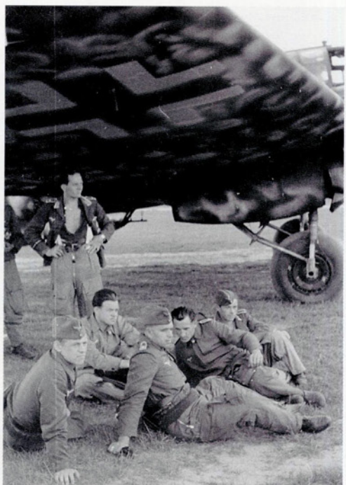
BELOW: A group of airmen wait beneath an He 111 H-11 (as indicated by the fore and aft guns in the ventral gondola). The Heinkel has black mottling over its pale blue undersides. The underwing cross is a type X and the mottling has impinged on it slightly. Also visible are the antennae of the FuG 101 radio altimeter. Guns both fore and aft in the ventral gondola indicate that this is an He 111 H-11. The open jacket and shirt of the Feldwebel standing on the right suggest spring or summer weather. (Note: almost certainly A1+AD, as in photograph above.)
