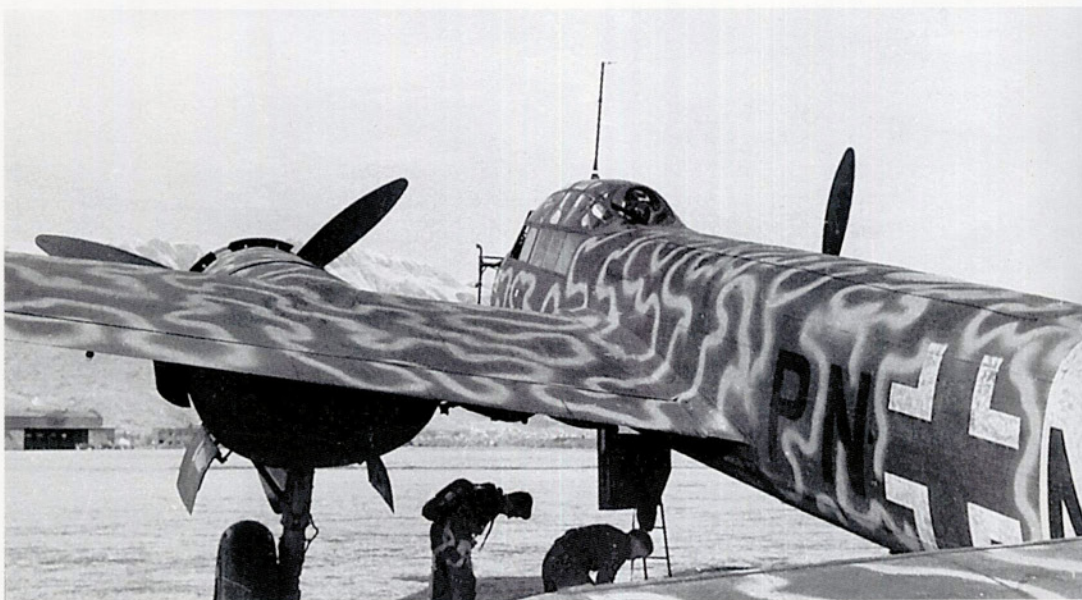
LEFT: Fitted with FuG 200 radar fitted to its nose this Ju 88 A-6, W.Nr. 4198 was operated by LG 1 from Aviano in northern Italy during spring 1944. The machine still carries the factory call sign PN+MT, although a white theatre band has been applied as well the scribble spray applied in RLM 65 as used effectively for aircraft flying over water.
