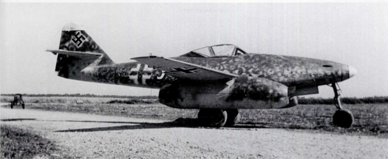
LEFT: Another Me 262 A-2a of I./KG 51, coded 9K+YH. This machine has two notable features. The first is that it carries two of the old ETC 503 type bomb racks, although they have a small timber fairing scribing them to the underside of the nose. The other is that the gun cowlings of the upper MK 108 cannon has had its gun ports blocked off, which was often done using some timber doweling and smoothing it into shape. On this occasion remaining two MK 108 gun ports have not been outlined in white.
