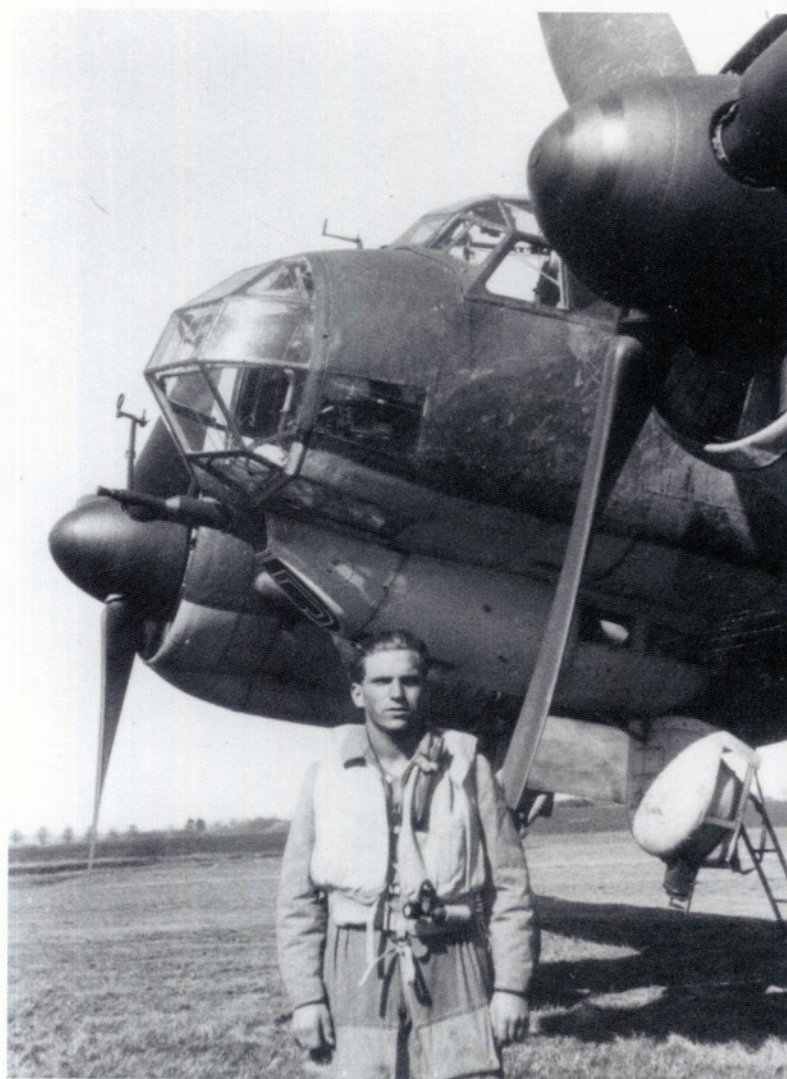
ABOVE: The 4. and 5./KG 77 spent the spring and summer of 1944 training at Heiligenbeil on the Baltic, as far as fuel supplies allowed. The original print of this photograph is dated '5/44.' This mud-spattered Ju 88 A (either a late A-4 or an A-14) is configured for torpedo-bombing: it has a 2 cm MG FF cannon in place of a bomb sight while painted on the sighting window is the aircraft's letter, a black or red 'J' with a white outline. There are three vertical lines painted on the nose glazing to assist the observer in lining up on a target. The camouflage appears to be the standard 70/71/65.
