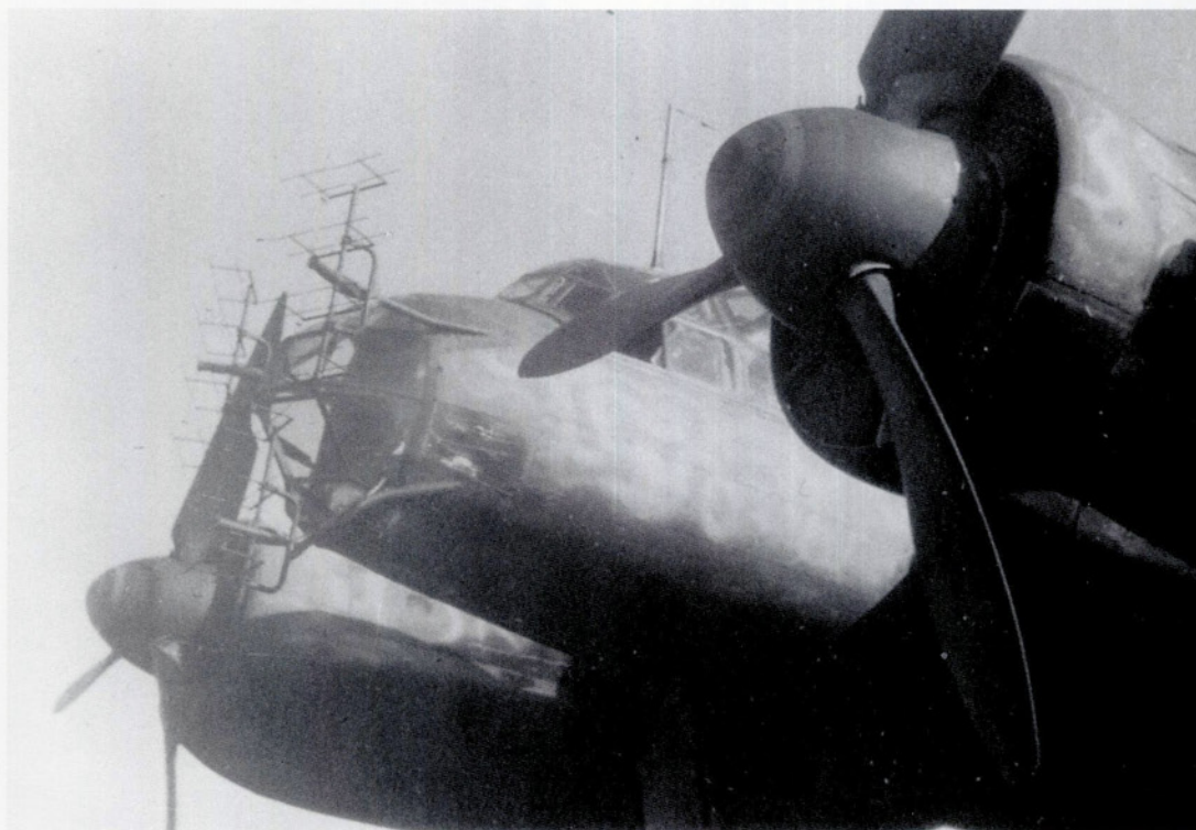
LEFT: Seen in the bright Baltic sunlight of May 1944, but destined for night operations, a Ju 88 A-17 of 4./KG 77, fitted with FuG 200 anti-shiping search radar and with no ventral gondola. The upper surfaces have been sprayed with a meander pattern of pale grey or blue over the basic greens and the undersides are black. The spinners appear to be black or dark green, with two red rings.
