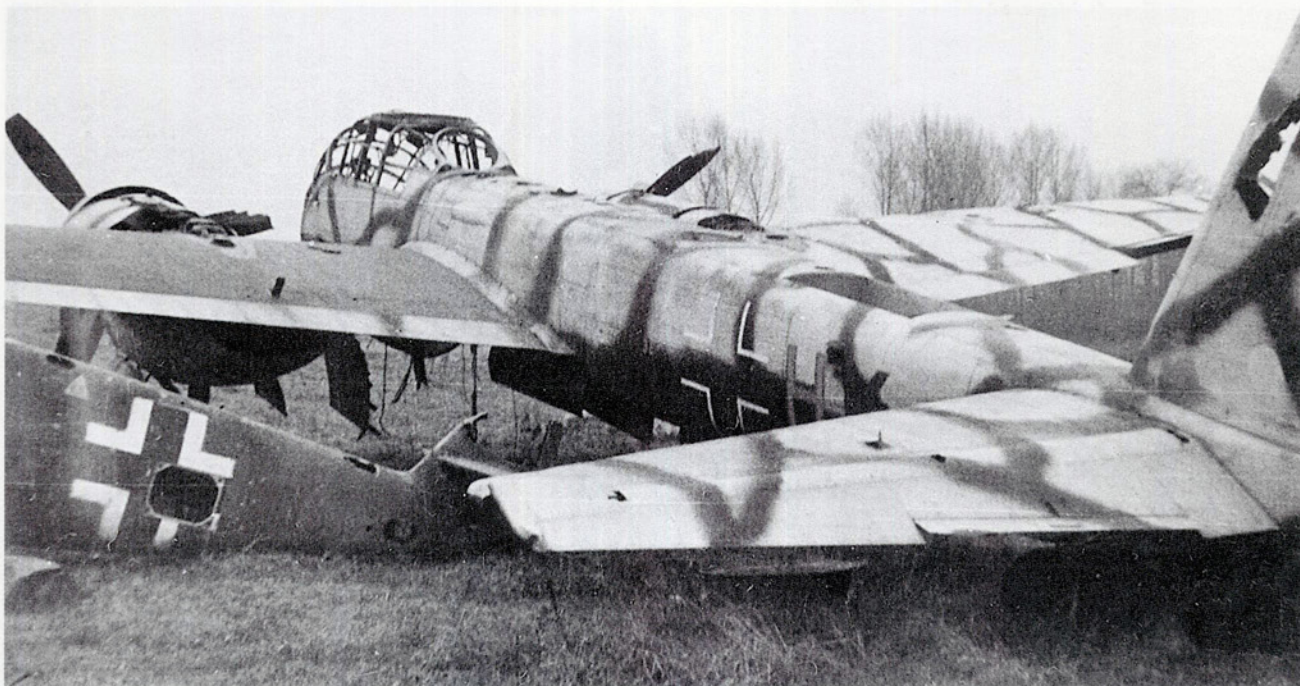
LEFT: This Ju 188 A-2 from 2./KG 6, coded 3E+HK, was found at Brussels-Melsbroeck in Belgium. The machine appears to be a hybrid, having at some time had its port wing replaced. The camouflage is typical of the late war schemes in being painted almost without any regard to standard finishes. The overall uppersurface finish appears to be RLM 76, which has been broadly oversprayed with either RLM 70 black-green or black.
