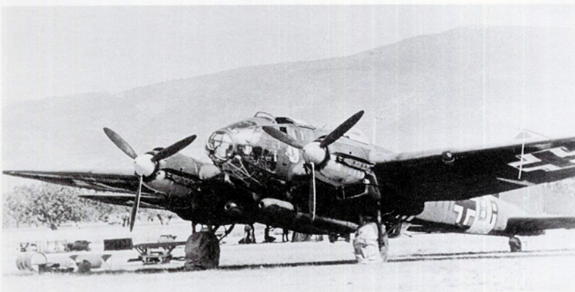
ABOVE: An He 111 H-6 converted to carry torpedoes belonging to 6./KG 26, stands ready for a mission on an airfield in Southern France. The aircraft is coded 1H+BP with the individual aircraft letter 'B' painted yellow on the wide white Mediterranean theatre fuselage band. The emblem of KG 26 is painted on the nose and on this occasion the spinners have also been painted yellow for the Staffel colour.
